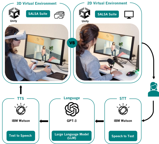
FIGURE 1. The high-level architecture of the child avatar system used in this comparative study also showing the two alternative interaction environments (2D vs. 3D).
