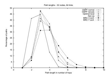
Fig. 12. Compares the backup path lengths of normal failure-free routing, OSPF full re-convergence (reroute), Optimal local (the best achievable path length for local recovery), Not-via and MRC with 3 and 7 backup configurations. We have used 100 Brite generated topologies with 32 nodes and 64 links.
