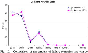
Fig. 10. Comparison of the amount of failure scenarios that can be covered by different IP Fast Reroute alternatives when using networks of different sizes.
