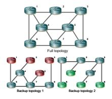
Fig. 11. Shows the original topology and how each node can be isolated once using 2 backup topologies.
