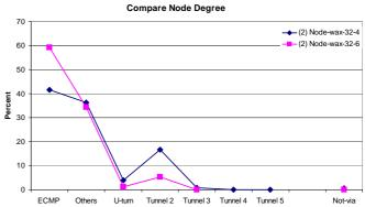
Fig. 9. Comparison of the amount of failure scenarios that can be covered by different IP Fast Reroute alternatives when using different average node degrees.
