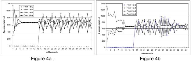
Scenario 2a with the Aggressive (4a) and the Reduce (4b) algorithm. The flow from 1 to 2 is not started until t=15 ms.
