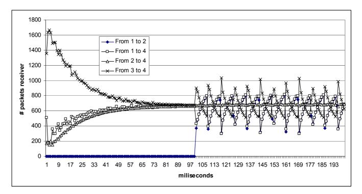
Figure 3. Scenario 2a with the Original algorithm. The flow from 1 to 2 is not started until t=100 ms.
