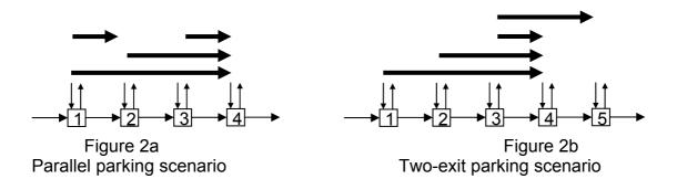
In the parallel parking scenario in figure 2a, the three flows into station 4 should share the bandwidth of  $I_{3-4}$  equally, i.e. they should get one third of the bandwidth each. If station 1 sends data to station 4 at one third of the full bandwidth of  $I_{3-4}$ , it may send data to station 2 at two thirds of the full bandwidth of  $I_{1-2}$ .
