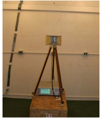
Fig. 17. Hardware experiment to validate the spatial spectrum generated by the ray-tracing tool.
