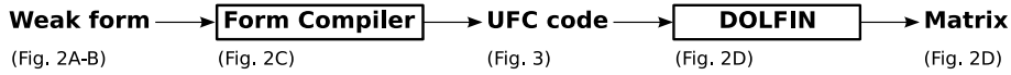
Fig. 1. Information flow from weak form of the PDE to global matrix assembly. The form compiler (SFC) takes a symbolic representation of the weak form and produces a C++ program which implements the UFC interface. This program is used as a computational kernel in the DOLFIN Assembler to produce the global matrix.
