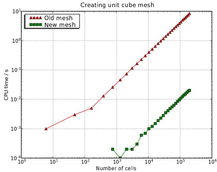
FIGURE 12. Benchmarking the CPU time for creation of a uniform tetrahedral mesh of the unit cube for the new mesh library vs. the old DOLFIN mesh library.
