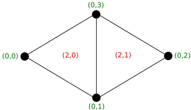
FIGURE 3. The mesh connectivity  $2 \rightarrow 0$  (the vertices of each cell) for this triangular mesh with two cells and four vertices is stored as two arrays `indices = [0, 1, 3, 1, 2, 3]` and `offsets = [0, 3, 6]`.
