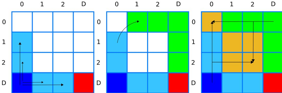
FIGURE 4. The three basic algorithms for computing connectivity. From the left: Build (computing connectivity  $D \rightarrow d$  and  $d \rightarrow 0$  from  $D \rightarrow 0$  and  $D \rightarrow D$ ), Transpose (computing connectivity  $d \rightarrow d'$  from  $d' \rightarrow d$ ) and Intersection (computing connectivity  $d \rightarrow d'$  from  $d \rightarrow d''$  and  $d'' \rightarrow d'$ ).
