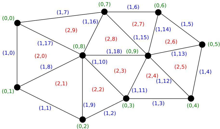
FIGURE 2. Each mesh entity of a mesh is identified with a pair  $(d, i)$ , where  $d$  is the topological dimension of the mesh entity and where  $i$  is a unique index for the mesh entity within its topological dimension, ranging from 0 to  $N_d - 1$  with  $N_d$  the number of entities of topological dimension  $d$ .
