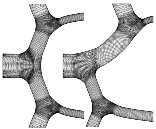
Grids are created from a parameterization, using custom written software
