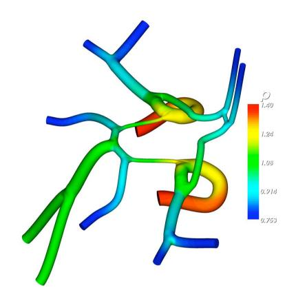
Using prescribed time varying flow rates on inlets, equal pressures on all outlets, and rigid vessel walls
