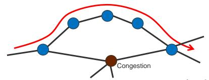
...look at adaptive routing as a supplementary mechanism to CC
