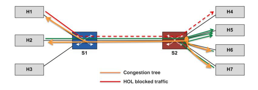
To avoid performance degradation, the HOL blocking must be removed.
