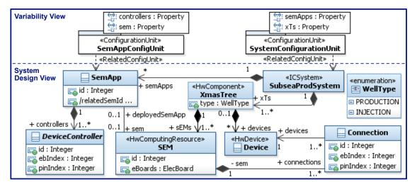
Figure 3: A fragment of the SimPL model for the subsea production system.
