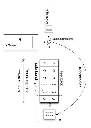
Fig. 1. SR ARQ and data-bundling Transmission Process
