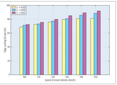
FIGURE 4. Comparison of edge caching hit rate with different vehicle speeds.
