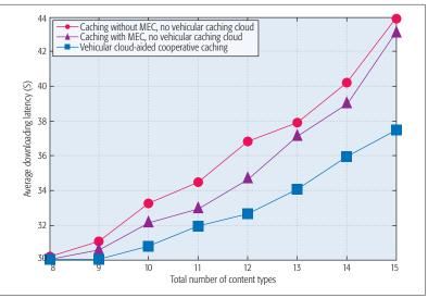
FIGURE 3. Comparison of content downloading latency of different caching schemes.
