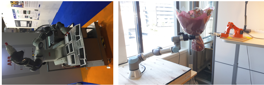
Fig. 1 Examples of collaborative industrial robots from ABB and Universal Robots (Picture credits: Arnaud Gotlieb, Mohit Kumar Ahuja).
