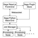
Fig. 3. Overview of the whole Saga platform, including how jobs are distributed for processing.
