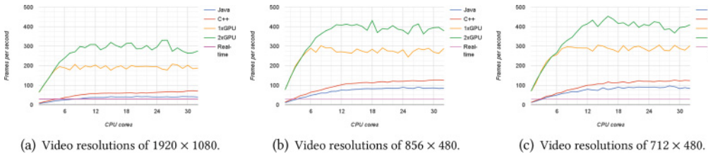
Fig. 4. The detection sub-system performance in terms of FPS depends on the number of CPU cores, the resolution of the videos, and the detection algorithm implementation.
