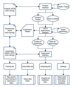
Fig. 3: GUI and JSON flow of GANEx
