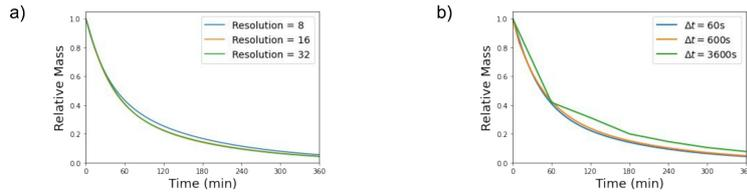
Figure 10: The evolution of total tracer mass relative to the initial value in the 7-compartment model, plotted for a) varying mesh resolution (with a timestep of 60s) and b) varying time step sizes (with mesh resolution 32).
