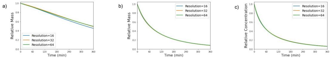
Figure 8: The evolution of tracer measurements relative to the initial value, plotted for varying mesh resolution. The simulations were run for a pure diffusion model using the tracer decay model and a time step of 1 minute. a) Relative mass within the entire brain. b) Relative mass within a cube with side lengths 2mm. c) Relative concentration at the injection point.
