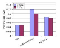
Figure 6: Power usage of system while running pipeline
