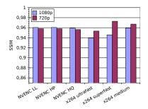
Figure 3: Video quality measured with SSIM.
