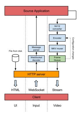
Figure 2: Block diagram of delivery pipeline
