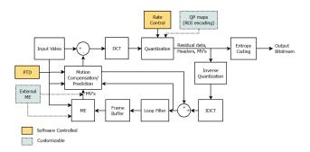
Figure 1: NVENC block diagram [3]
