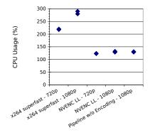
Figure 7: Total CPU usage of delivery pipeline
