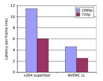
Figure 5: Latency of encoding a single image
